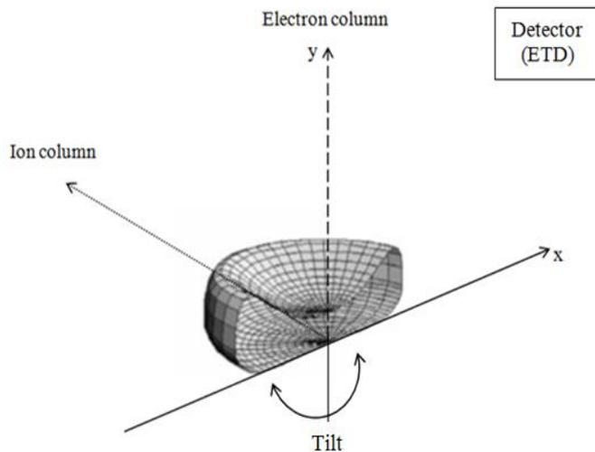
**Figure 5.** Scheme of the orientation of the ion and electron columns in a FIB/SEM, applied to the Euclid's Optics theorem XXXVI. The electron column is set on the Y axis, perpendicular to the sample (X-Z plane); the ion column is set on the X-Y plane, at a fixed angle (52°) compared with that of the electron column. In this scheme Euclid's wheel has been replaced by a RBC, and the two primary particle beams play the role of the light source in an usual vision process (optics). The
